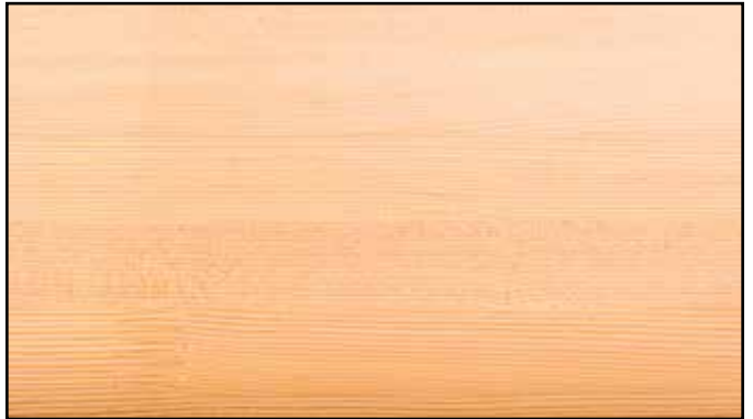
Douglas fir vertical grained, finger jointed glulam timber.
