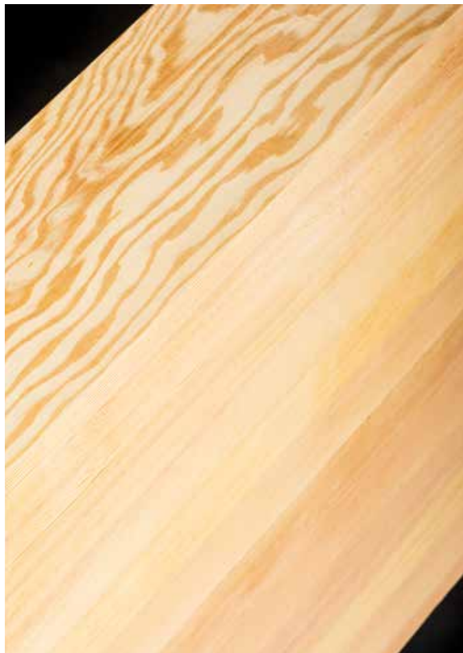
Top of Douglas fir EdgeMatched glulam showing flat-sawn grain on the narrow face with edge grain on the wide face creating a more natural appearance.
