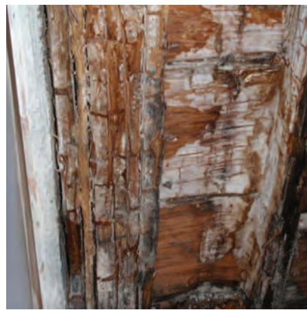
Figs. 5–7 From left, brown rot in timber, white rot in house trim and sapstain in newly manufactured lumber.
